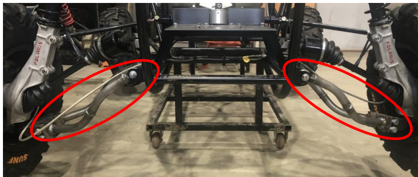
Figure 11 - Front Control Arm Alignment
