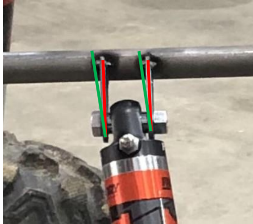
Figure 12 - Rear Suspension Support Alignment
