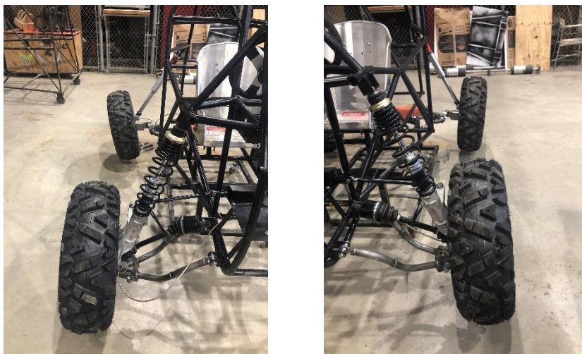
Figure 13 – Left and Right Camber Difference
