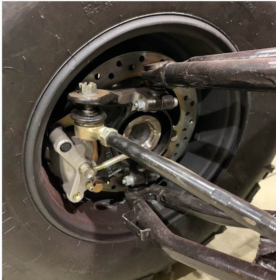
Figure 14: Brake line connecting to caliper
