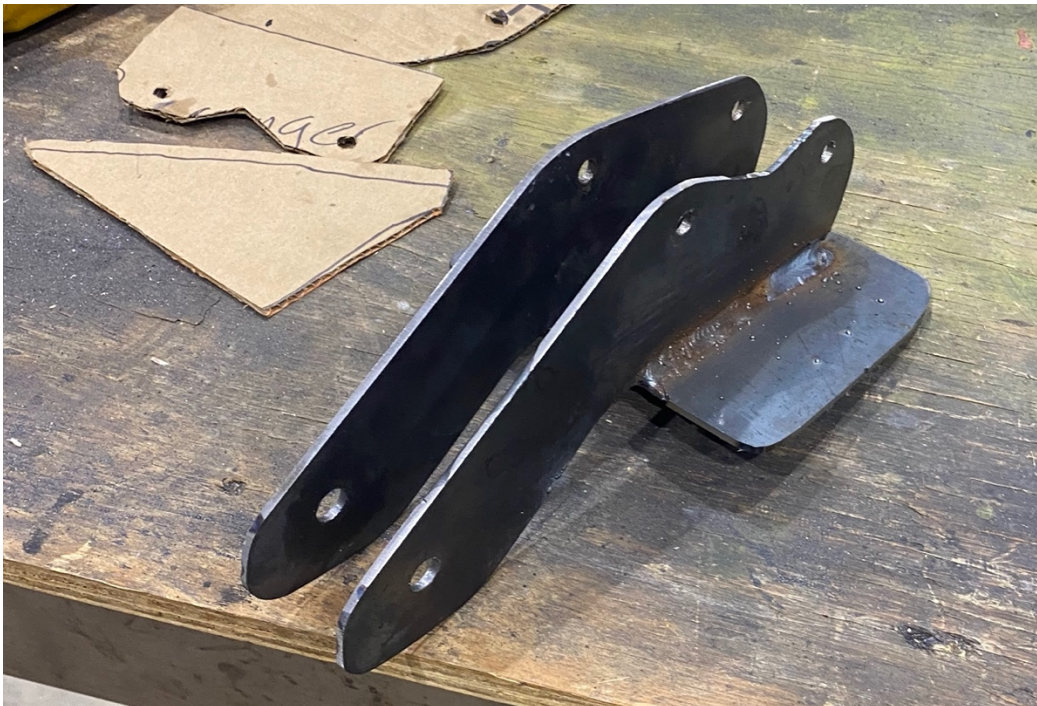
Figure 13: Paddle and Master cylinder mounting bracket
