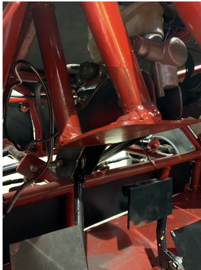
Figure 15: Master cylinder and Paddle assembly with brake lines
