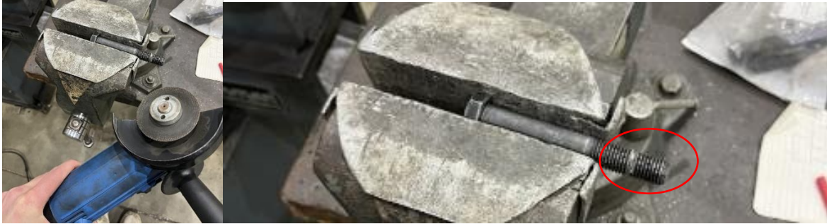
Figure 78: Cutting the Weapon Shaft to Length Using an Angle Grinder
