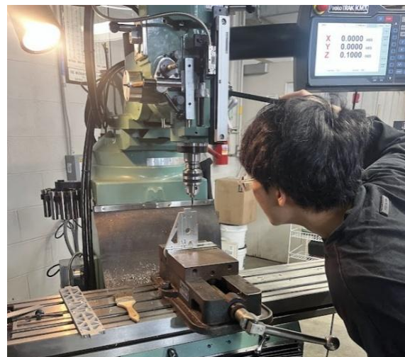
Figure 71: Drilling Holes with End Mill
