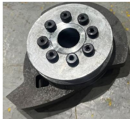
Figure 80: Completed Weapon Stack-up Assembly
