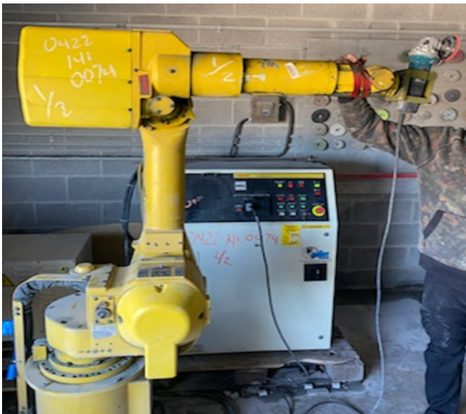
Figure 18: Assembly of EOAT & S-10
