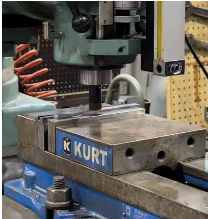
Figure 41 – Milling outer edge for correct width/height and to ensure it's perfectly flat.
