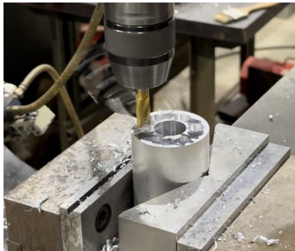
Figure 47 – CNC drill pressing screw holes and counterboring for screw heads
