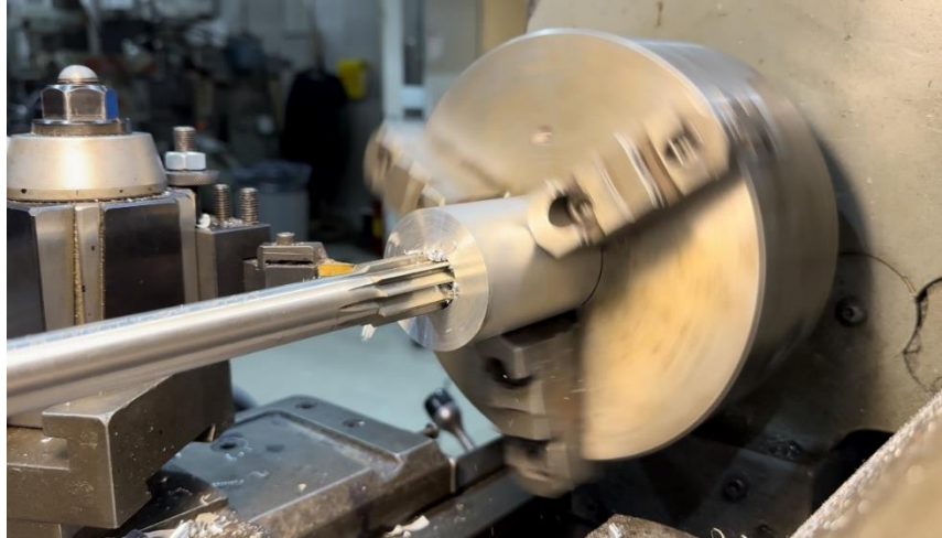
Figure 46 – Drilling out and reaming 15/16” Hole
