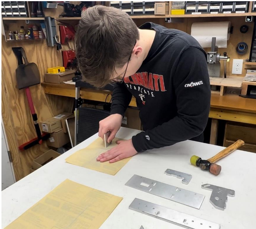
Figure 34 – Sanding down the oxide layer
