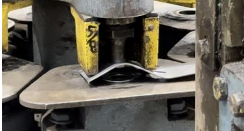
Figure 45 – Punching washer for correct ID before cutting on the vertical band saw.
