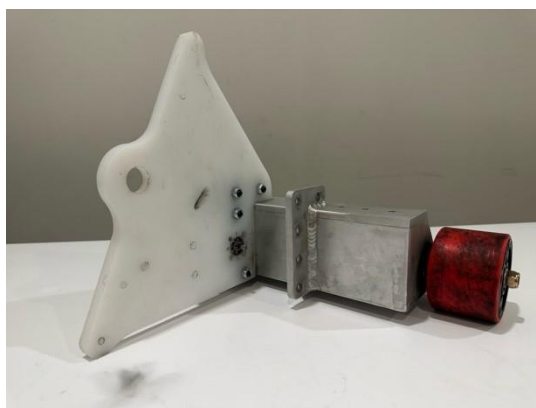
Figure 65 – Step 3: Attach first upright to chassis and slide on weapon motor shaft bearing.
