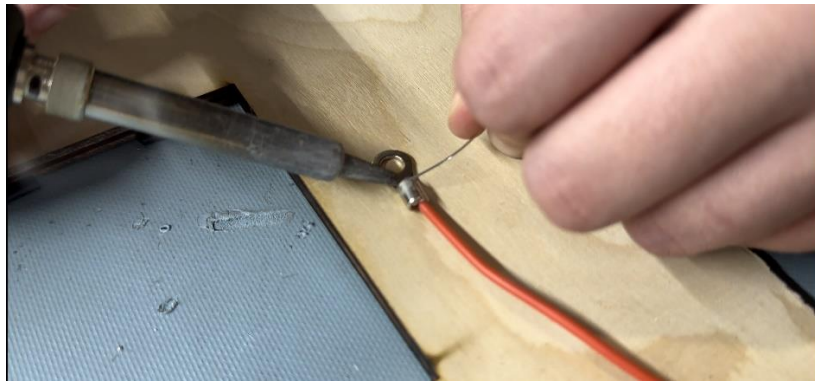
Figure 53 – Soldering example showing the addition of eyelet connectors.
