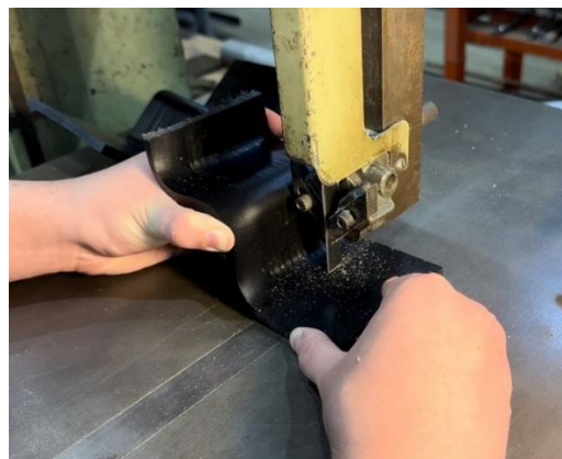
Figure 59 – Cutting off excess material before drill pressing holes for connection points with the uprights and chassis.
