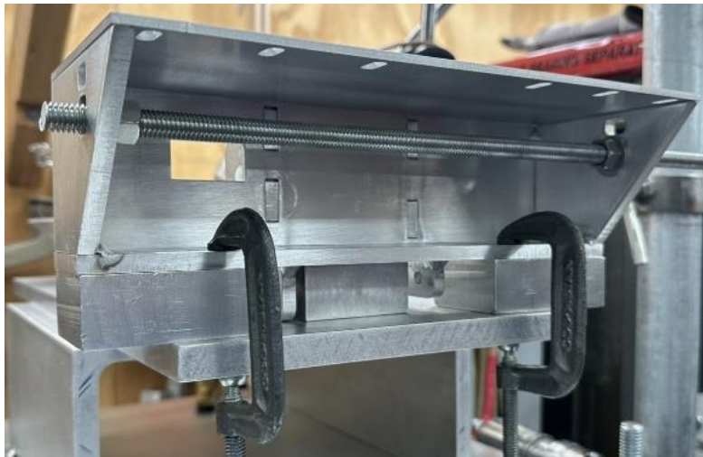
Figure 39 – Clamped setup to ensure no offsetting during the welding.
