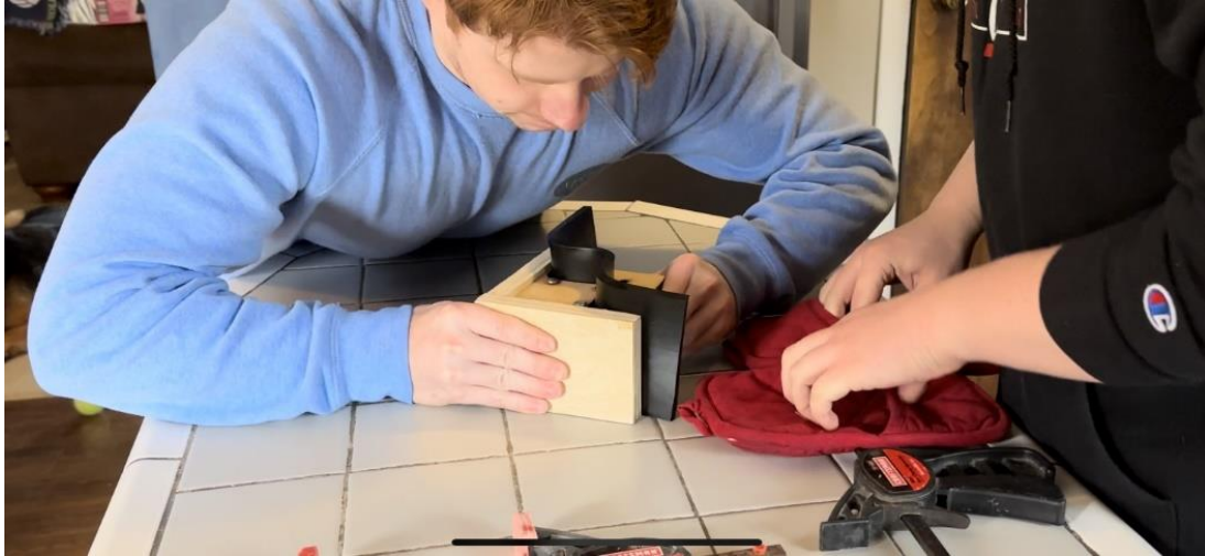
Figure 57 – Pressing UHMW to desired shape at 10 degrees below its melting point.
