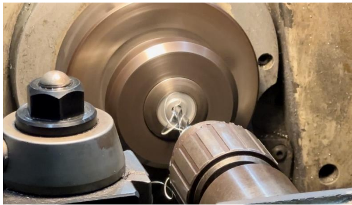
Figure 50 – Drilling on lathe for correct ID on pulleys
