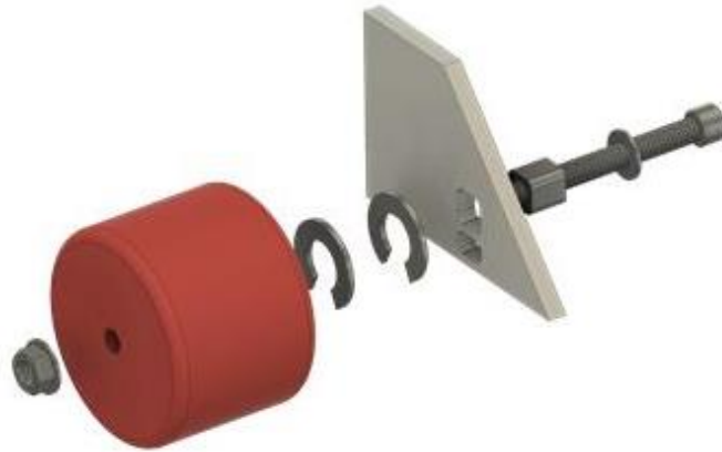
Figure 26 – Wheel Assembly Including the Steel Locking Part
