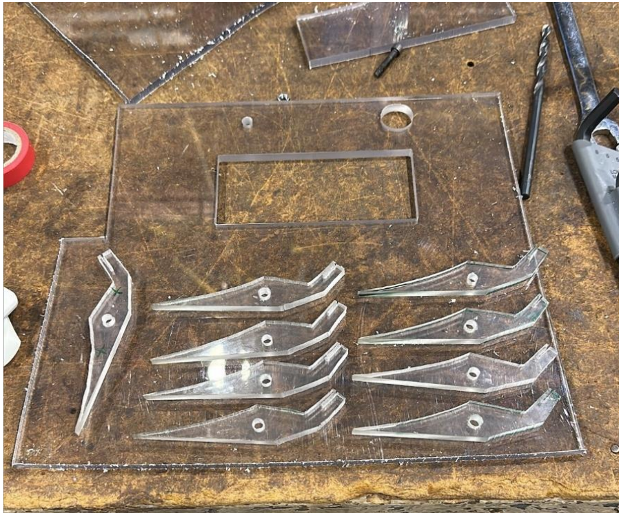
Figure 61 – Hand cut polycarbonate forks using a vertical band saw and drill press.
