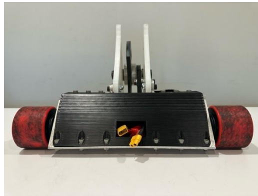
Figure 71 – Step 8: Tighten down backing and have battery plug sticking out for easy access.
