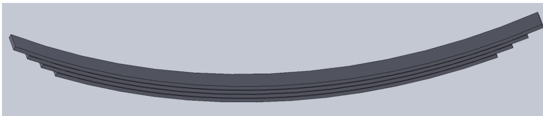
Figure 4: Altered size leaf spring concept 2
