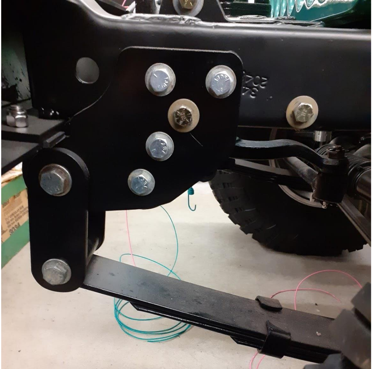
Figure 14: End mount for front driver side leaf spring
