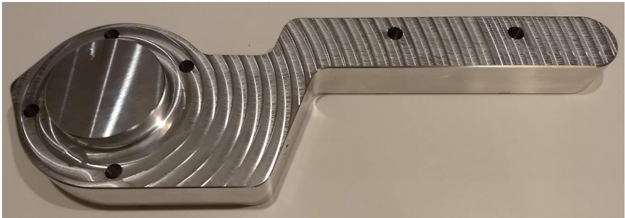
Figure 9: Bottom contour of e-brake bracket
