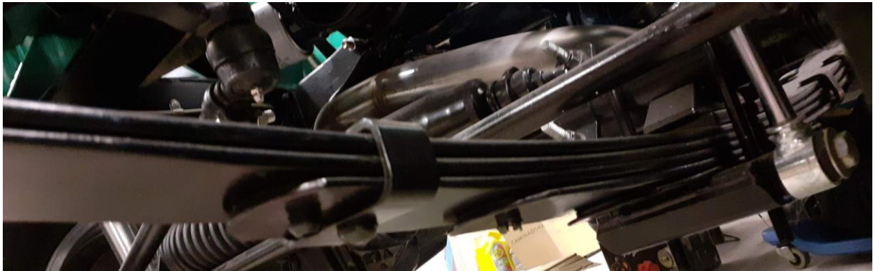
Figure 13: Axle mount for leaf spring
