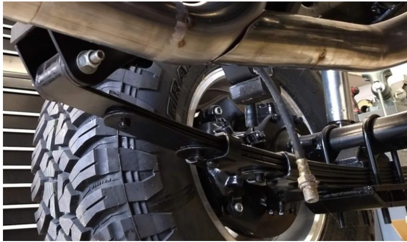
Figure 12: Inside mount for front driver side leaf spring
