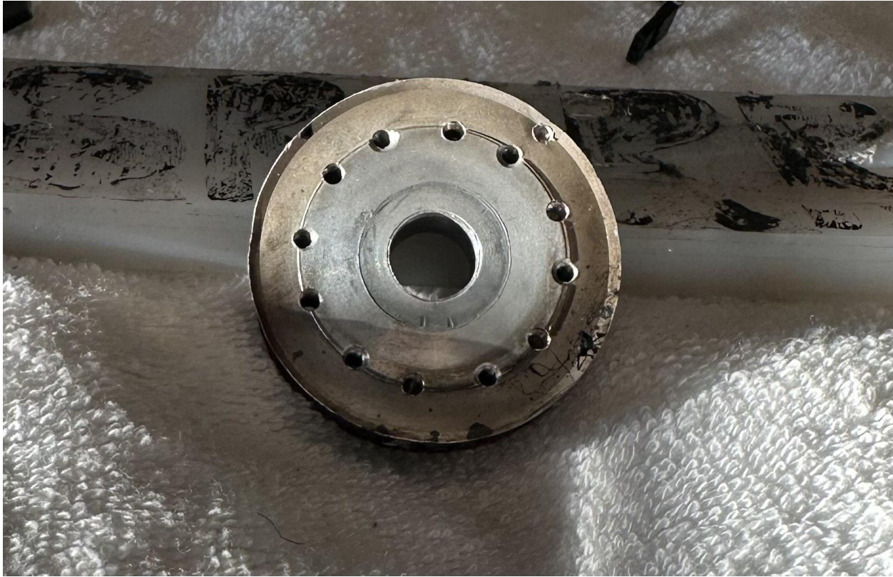
Drilled and Tapped Weapon Stack Pulley
