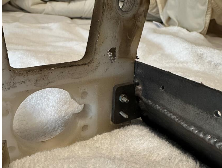
Welded Tab on Plow Connecting to Upright
