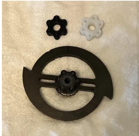
TPU Weapon Spacer installed on Spinner
