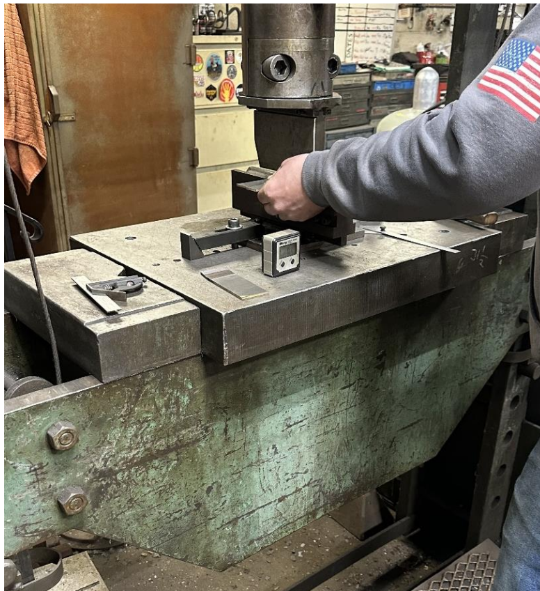
Hydraulic Bending of Front Plow
