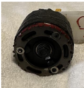
Titanium Cleats on Wheels with Limited Clearance
