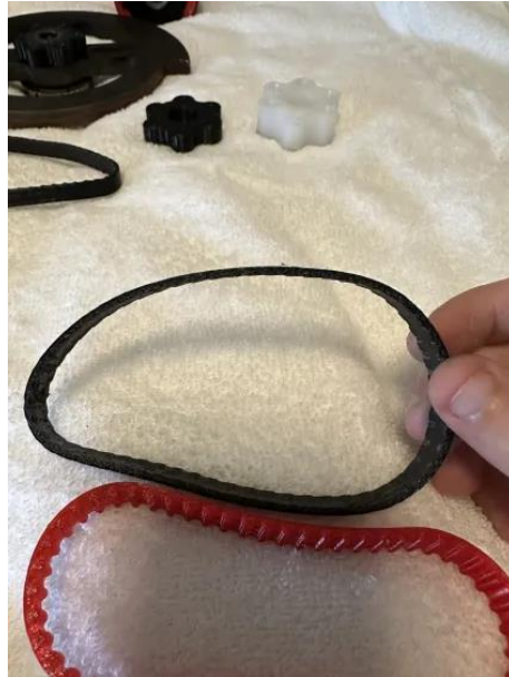
TPU Belt with Worn Down Teeth
