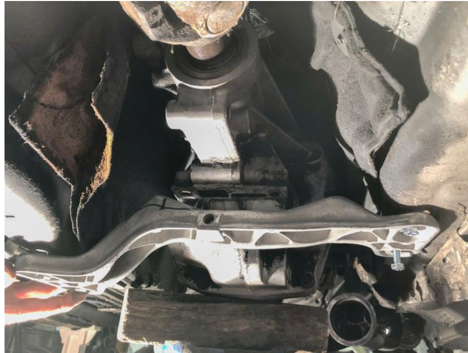
Figure 1.8. Original Automatic E36 Transmission Mount Installed
