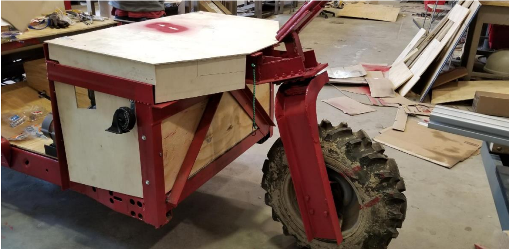
(Figure 10) Completed front engine housing with guards.
