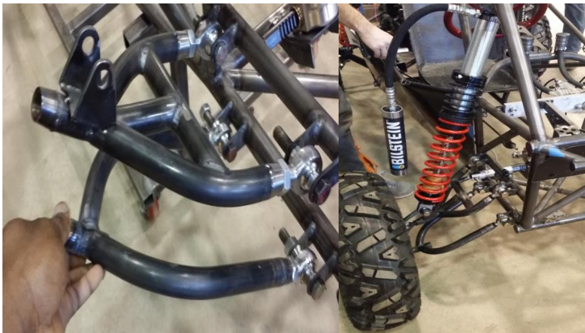
Figure 14: Control arms &amp; shock mount
