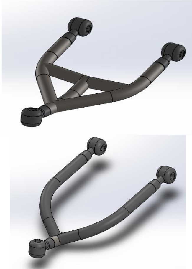
Figure 9: optimized upper Arm and Lower Arm
