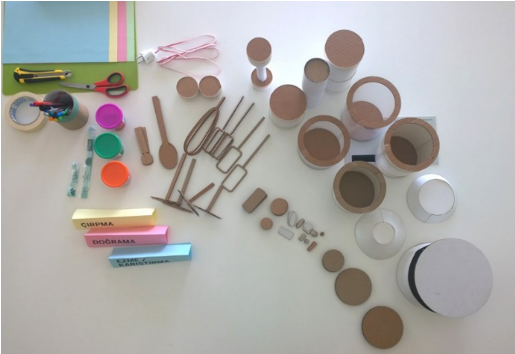
Figure 3. An example of the ERM toolkit prepared for blender/mixer product category including laser-cut parts and additional materials
