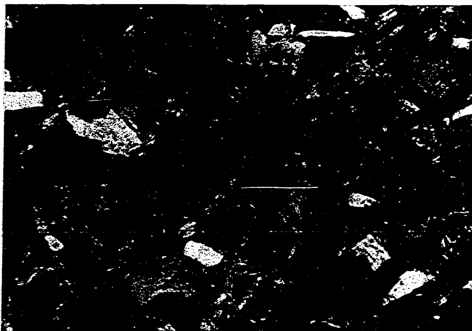
FIGURE 13. Photomicrograph of sample KB-6B with an angular and fresh quartz grain (grayish-brown) at lower left. Sample consists mainly of abundant biotite flakes (brown) and alkali-feldspar crystals (gray) in an altered, micaceous and clayey matrix (x nicols, x 2.5).
