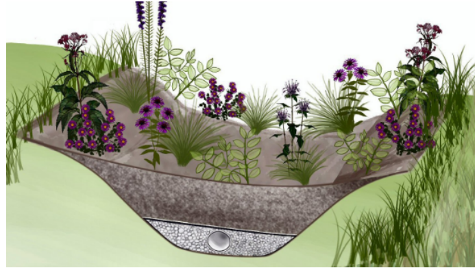
Figure 1: Bioswale Cross-Section (Source: Vegetated Swales, 2022)
