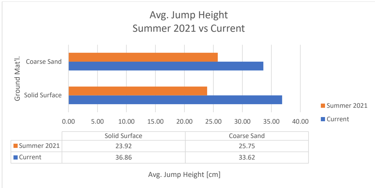
Figure 21: Average jump height, in centimeters, compared between the last iteration of the fixture and the current
