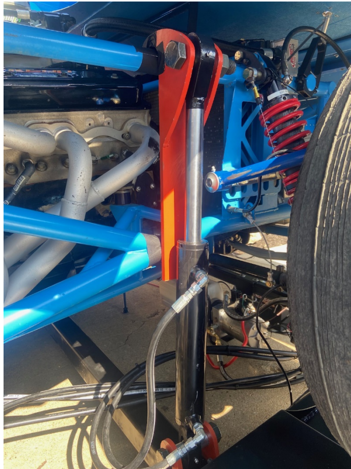
Fig. 8: Completed Right Front Bracket
