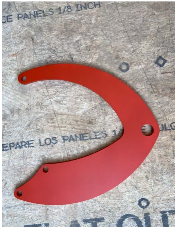
Fig. 10: Completed Lift Bar Plate
