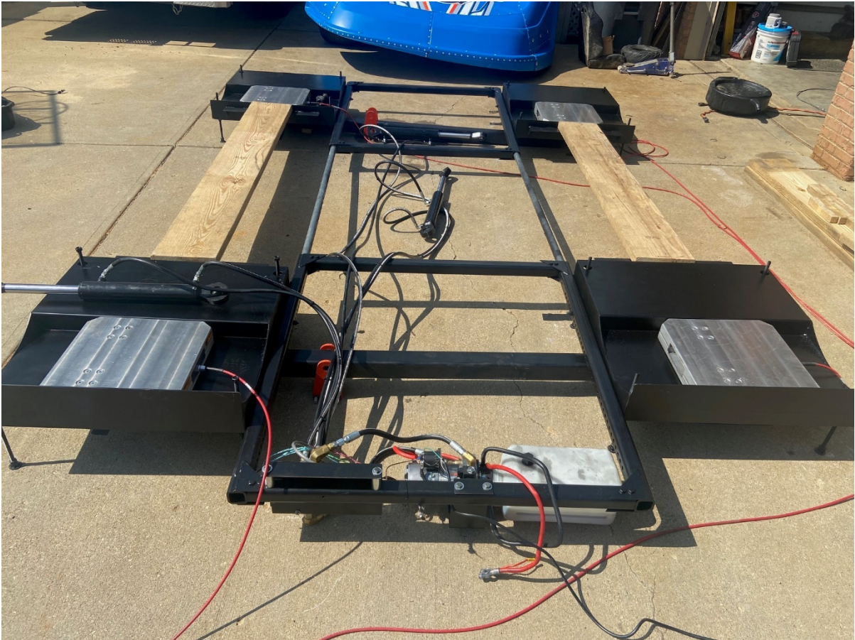
Fig. 11: Final Assembly of Pull-Down Machine
