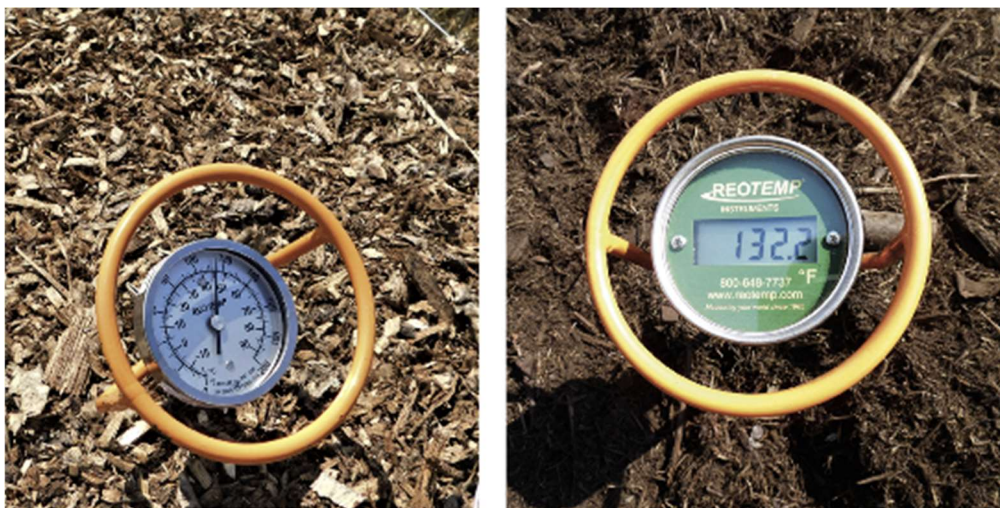
Figure 20: Bimetallic thermometer with a dial readout with its orange handle (Rynk et.al. 2022)
