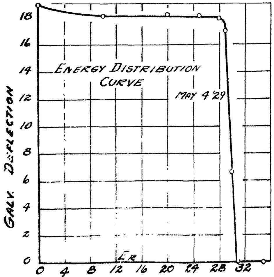
apparatus, served to determine the energy distribution of the beam. Typical energy distribution curves for this apparatus, as well as for the previous arrangements, are shown in Figures 4 and 5. The diameter of the circular opening,  $O$ , is one centimeter. Therefore a spot of 1 cm. diameter is irradiated with electrons. This is larger than the area that could be irradiated with the first apparatus.
