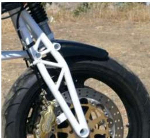
Figure 5: Hossack Suspension design on motorcycle
