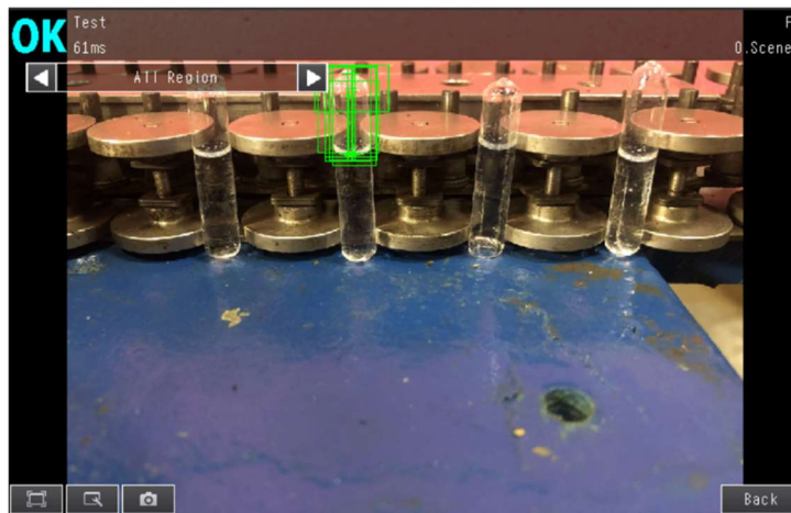
Figure 2 - Sensor detecting an 'OK' Ampoule
