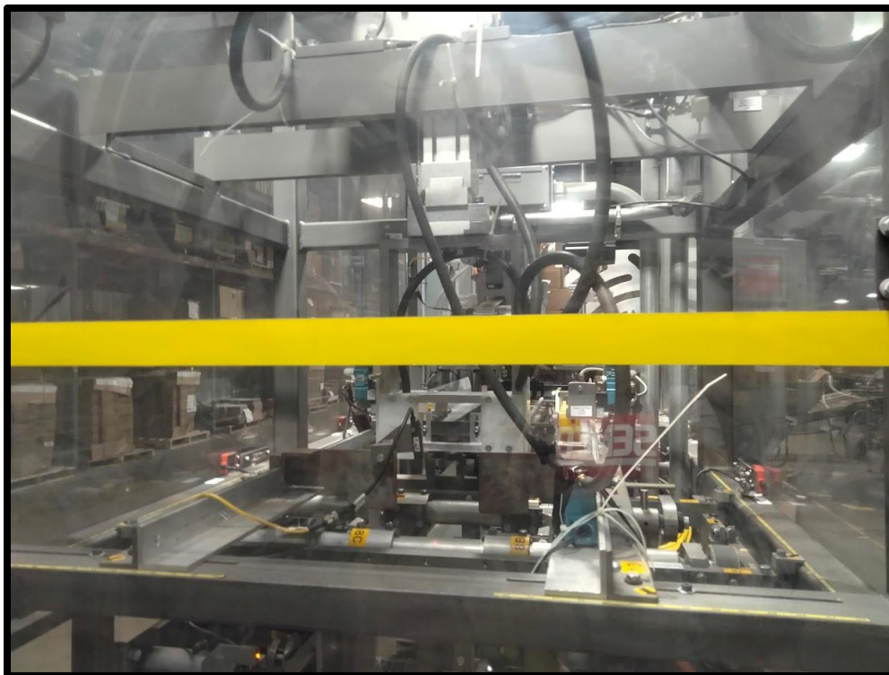
Figure 28 – Air hose connections from vacuum tank to suction cups through the solenoid, machine front
