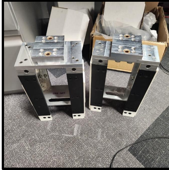
Figures 21a-21c – Images of fully assembled mandrels for NM 2501 & 2507 (left) and NM 2508-2511 (right) – In figure 21b (top right), both mandrels have had their respective carton models laser engraved on. This is also the case for the mandrel in figure 20a & 20b.
