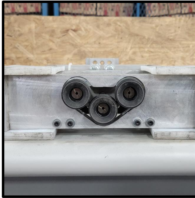
Figure 26 – Underside view of NM 1670 mandrel with suction cups
