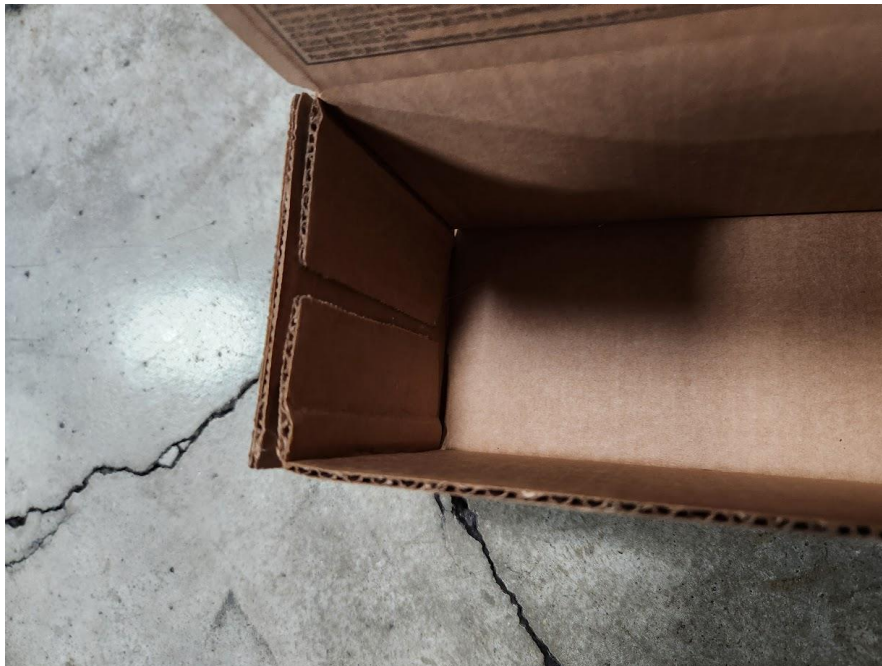
Figure 39 – Image example of crinkles on the inside of the carton
