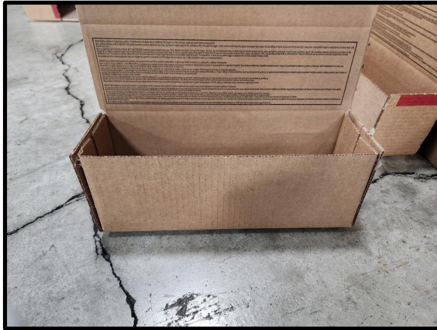
Figure 38 – Image example of minor flap separation (evident at sides)
