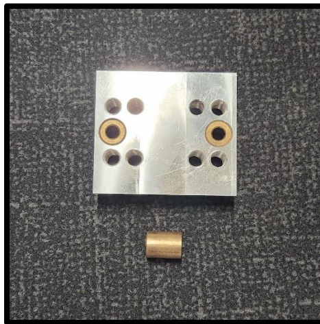
Figure 22 – Stock length brass bushing and result after cutting and pressing into mandrel arm attachment - 3 of this item was made for each respective mandrel
