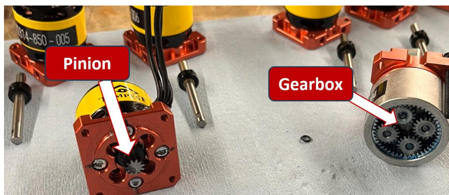
Figure 7.3.02 Disassembled Gearbox & Motor
