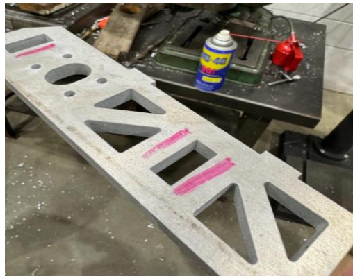
Figure 7.1.05 Missing Holes on Frame
