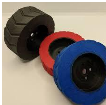
Figure 1.10: Rubber Resin Poured Wheels
