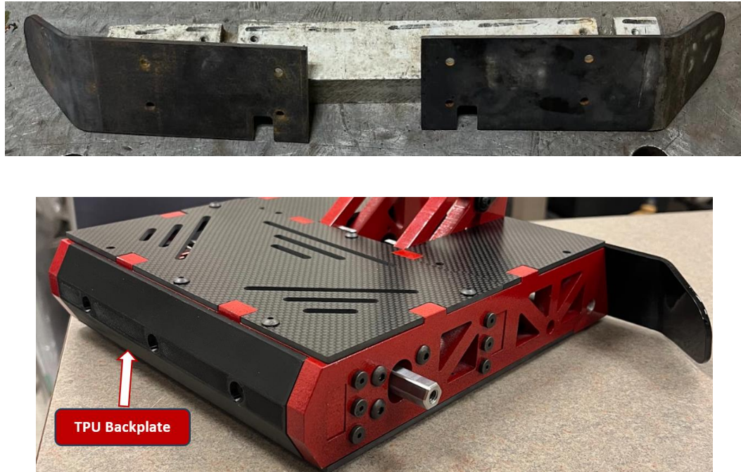
Figure 7.1.08 Plows & Rear Armor
