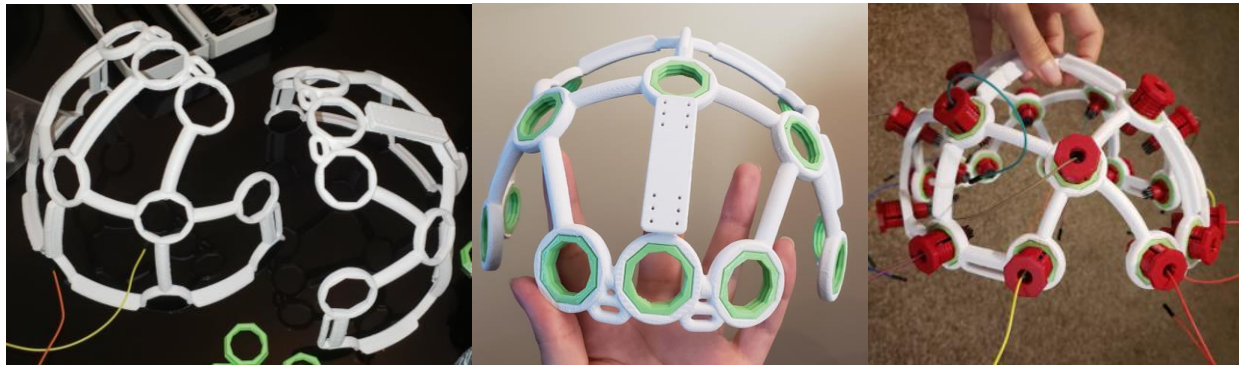
Figure 7 - Headset Build, UltraCortex III 3D Printed Frame
