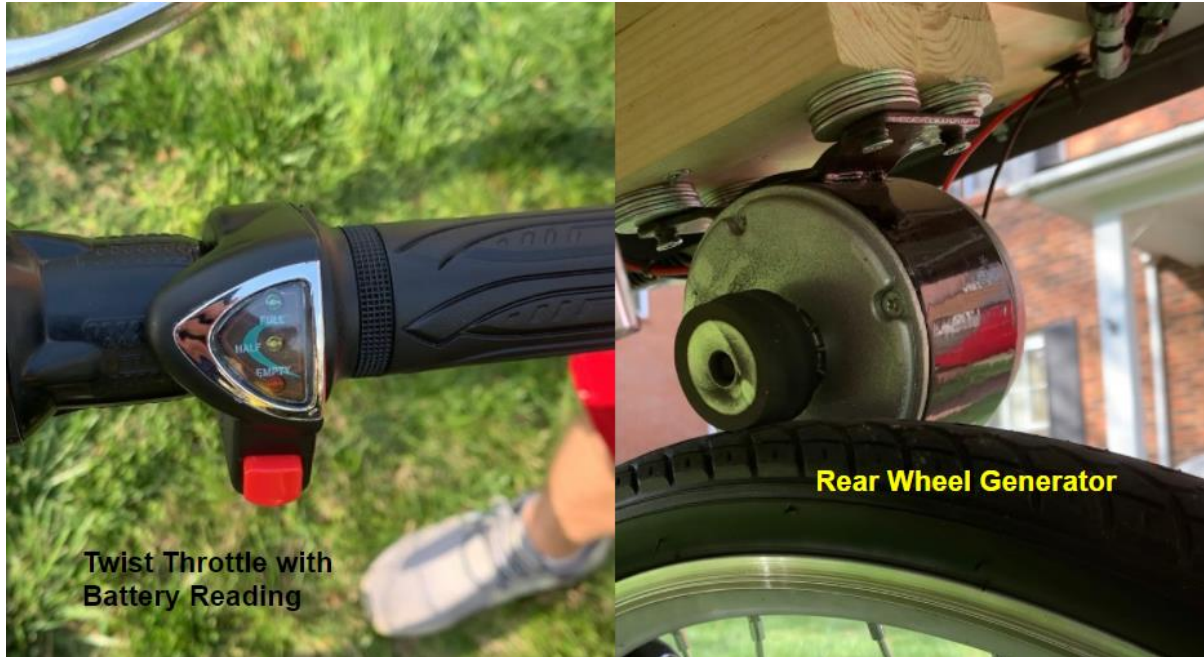
Figure 18: Twist Throttle and Rear Wheel Generator
