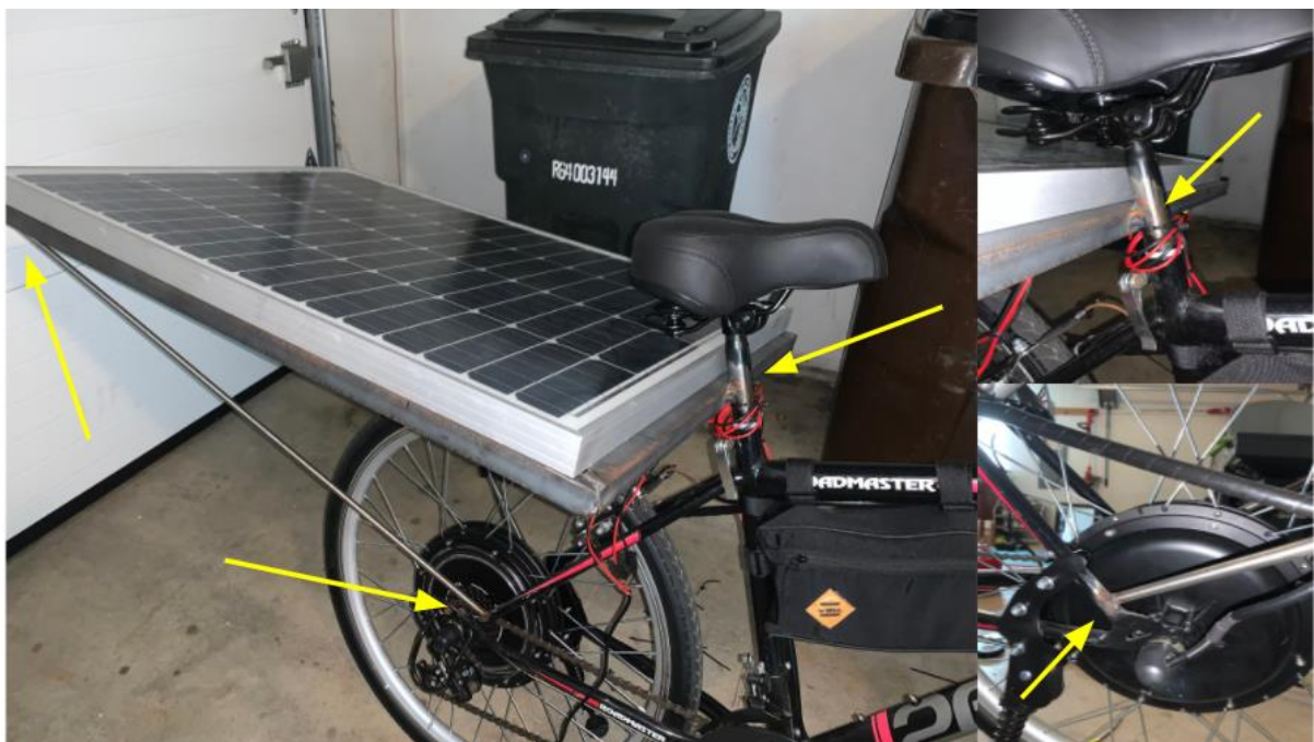
Figure 16: Welding Points for Solar Panel Frame
