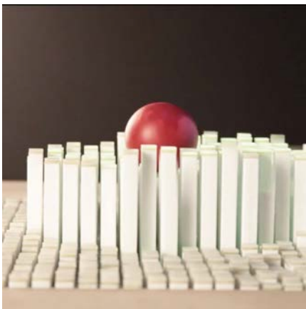
SMALL PEGS RISE AND FALL TO CONTROL THE BALL
