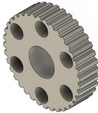
Figure 43: 32-tooth weapon pulley
