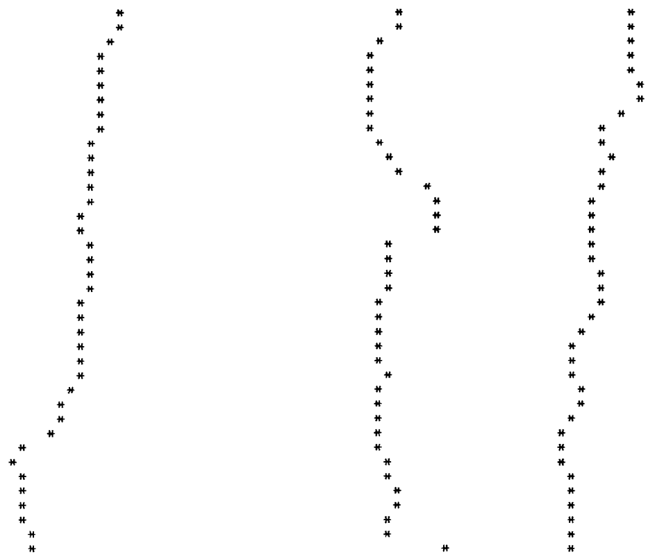
PORE TORTUOSITY MAP; THREE FLOW PATHS APPROXIMATELY PARALLEL TO COLUMNS (MODIFIED METHOD OF PRESTON AND DAVIS, 1976)
