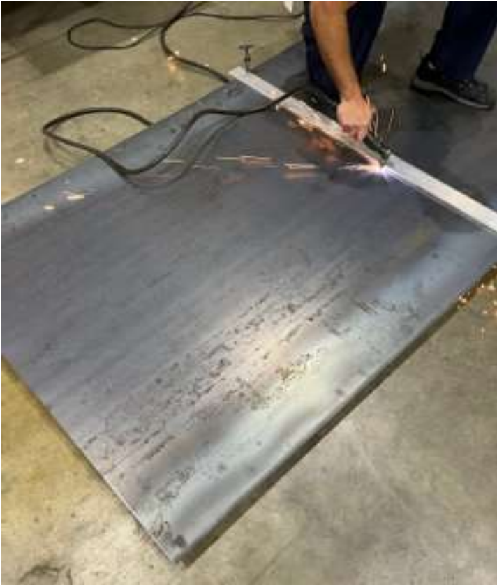
Figure 45: Plasma cut flooring
