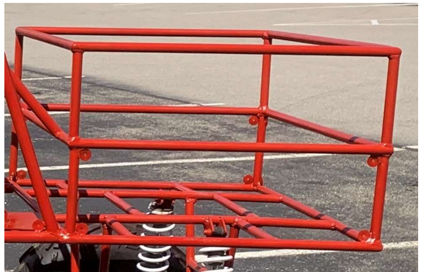
Figure 54: Finished bed mounting
