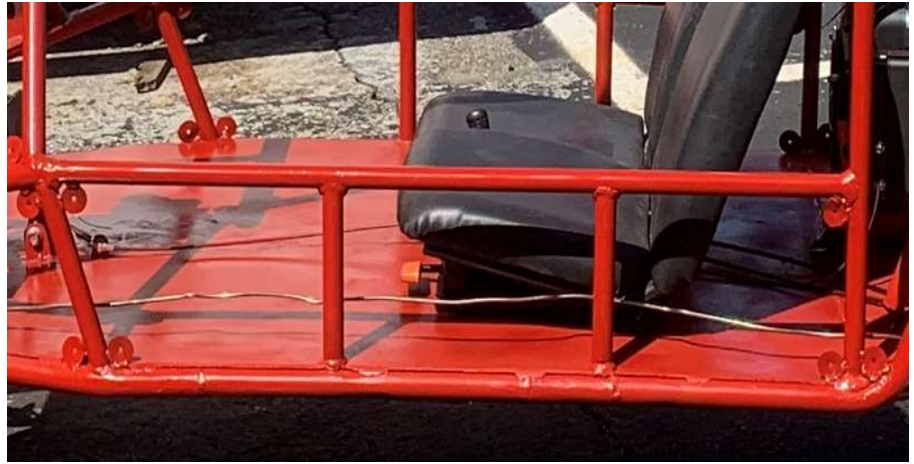
Figure 48: Vertical Bracing bars
