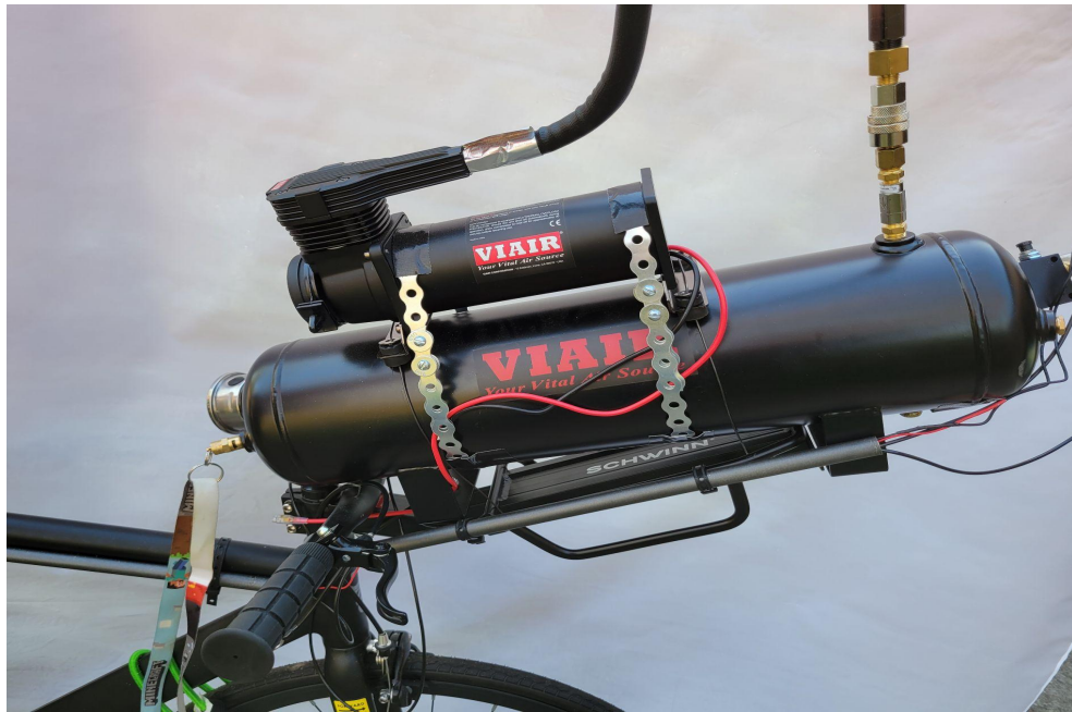
Figure 19: Profile of Tank Setup at side view
