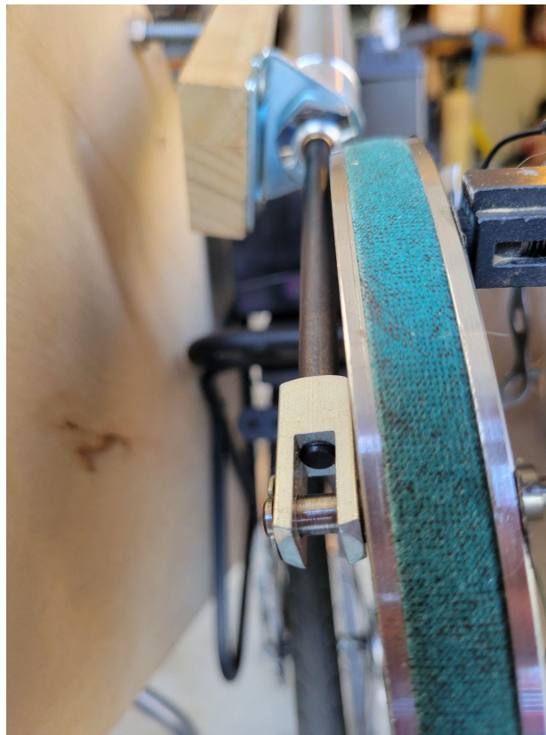
Figure 22: Warpage from the Threaded Rod
