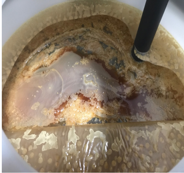
Figure 1.2. shows the skimming that is occurring in the day-tanks
