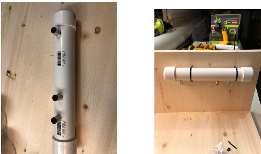
Figure 1.12. the images above shows the drilled and tapped holes on the PVC pipe
