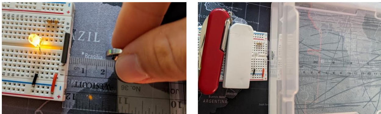
Figure 8: Reed Switch Test Setup
