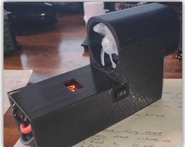
Figure 14: SolidWorks Housing Design and 3-D PLA Print
