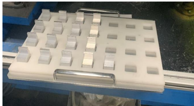
Figure 13: Fabrication of Tray Design 1 – Part D3225
