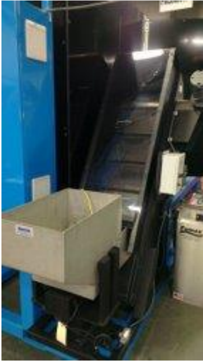
Figure 1: Hopper & Incline Conveyor
