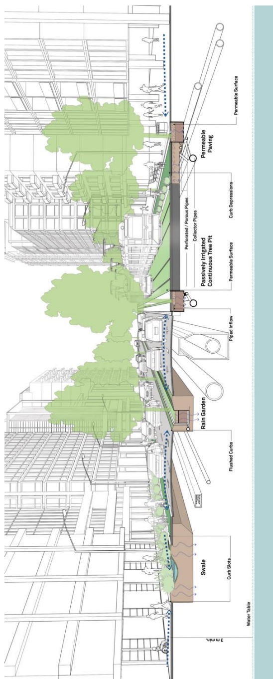
Figure 5. A visual representation of potential horticultural and green infrastructure that can assist in managing stormwater in the urban landscape (Green Infrastructure and Stormwater Management 2022).
