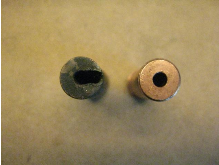
Figure 1, Left worn tip, right unused tip. Both are 3.2mm tips, both show the exit side of the tip
