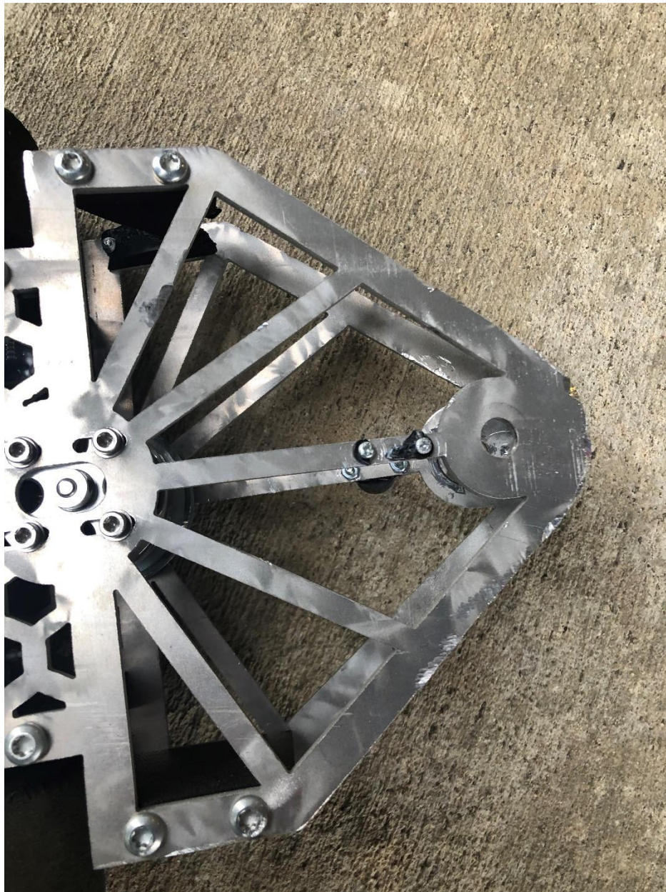
Figure 52: Underside Frame Damage
