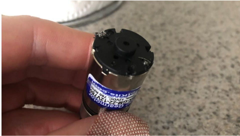
Figure 49: DC Motor with Missing Leads
