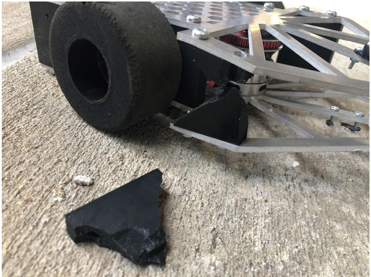
Figure 57: Broken Side Wall
