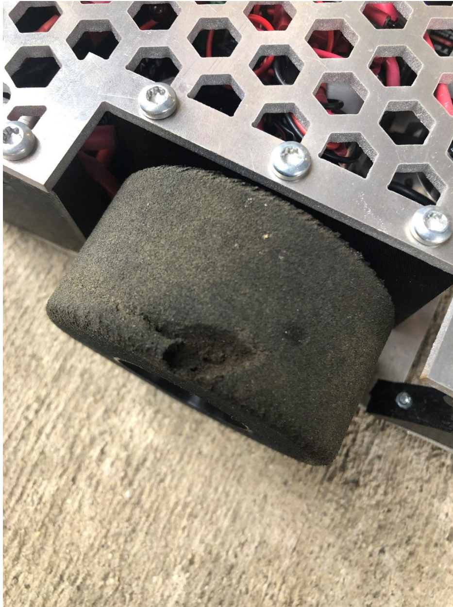
Figure 54: More Wheel Damage
