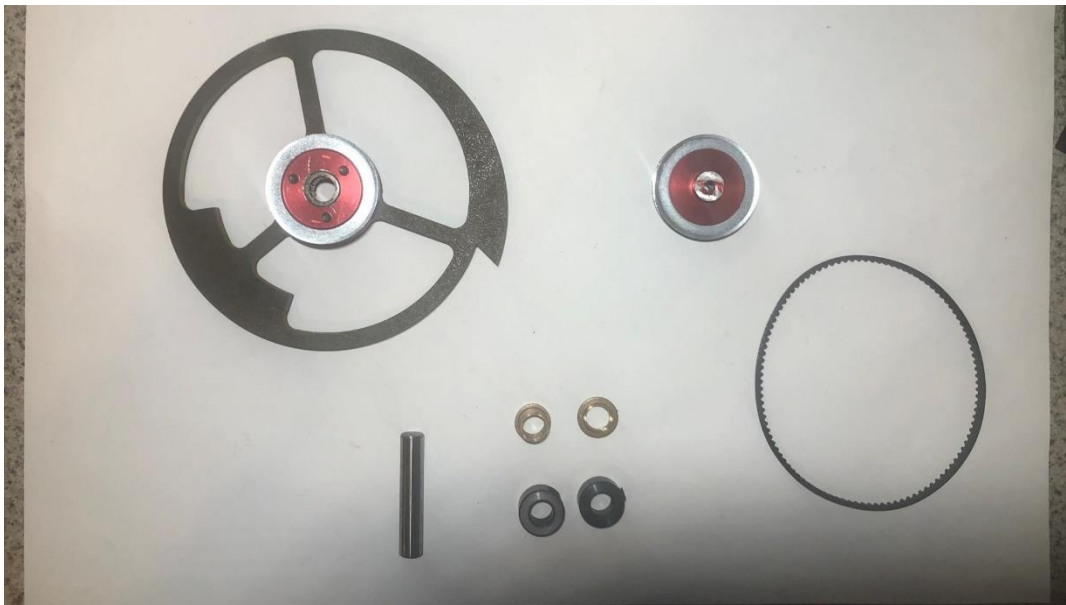
Figure 39: Components: AR500 Blade, Weapon Shaft, (2) Collars, 42T Pulleys, 107T Belt
