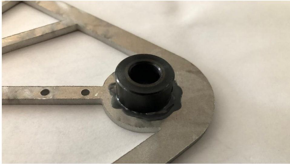
Figure 51: JB Welded Shaft Collars Attached to Frame
