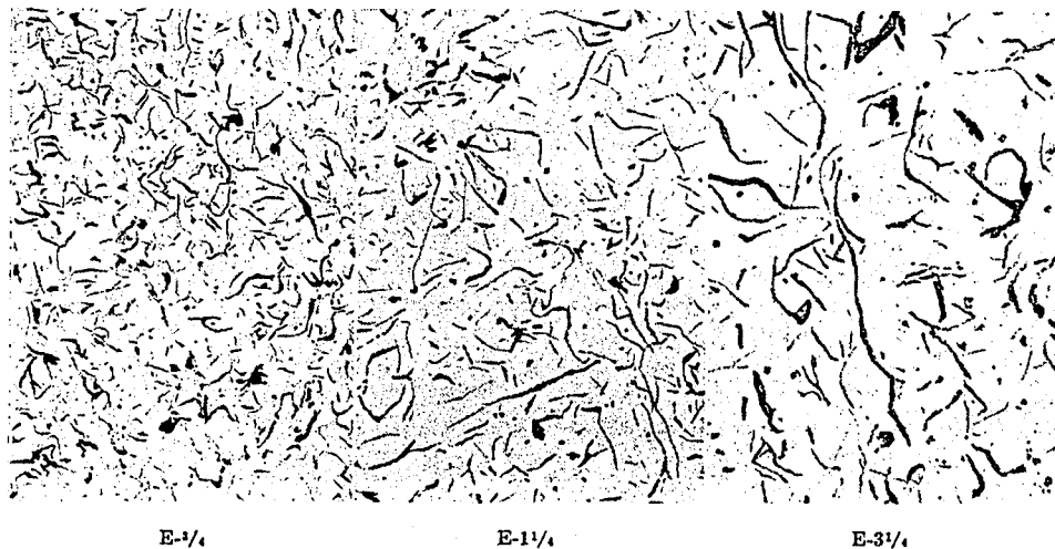
Fig. 1 PHOTOMICROGRAPHS OF GRAPHITE DISTRIBUTION (Unetched; \times 50 .)
