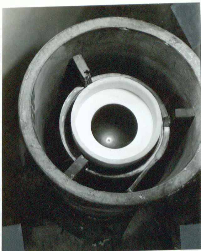
Fig. 30. Furnace viewed from the top with the alberene lid off.
