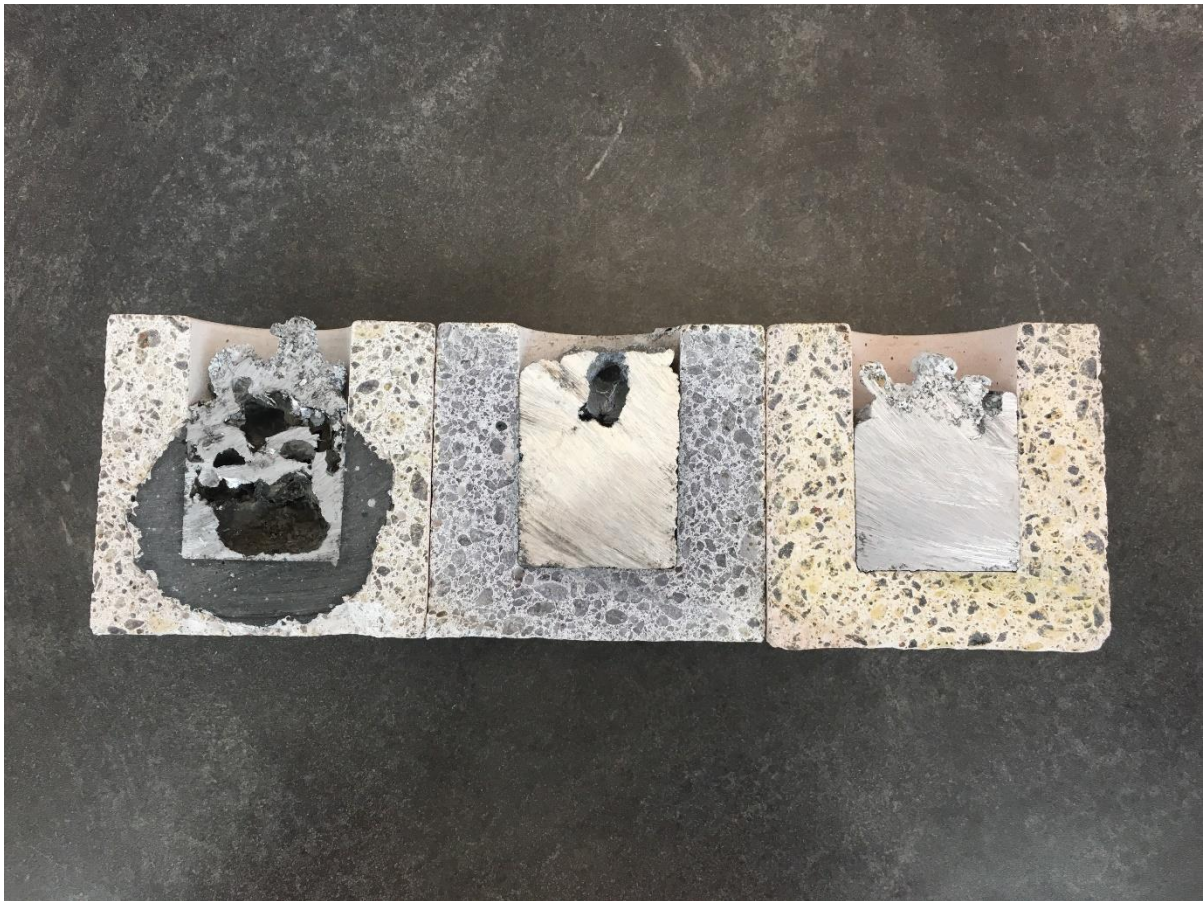
Figure 1: Refractory testing. Left to right: Cement, IPSX, ASX-60 Al-MG
