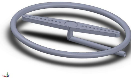
Figure 1: Single spray arm with internal heating ring
