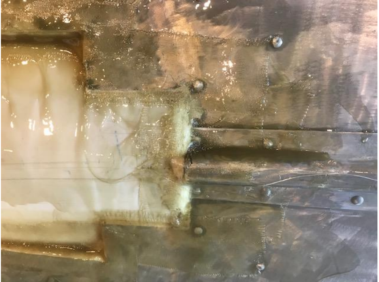
Close-up to show consistency of dried fiberglass.
