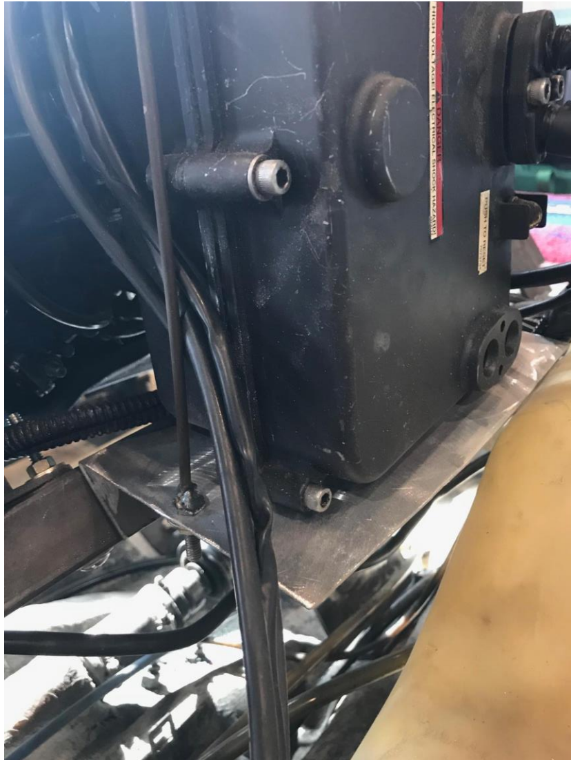
Repurposed aluminum panel from boat seats bolted to engine frame to support CPU box.
