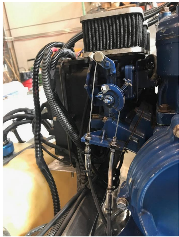
Salvaged throttle from 70s Chris Craft to control reverse bucket and gas throttle.
