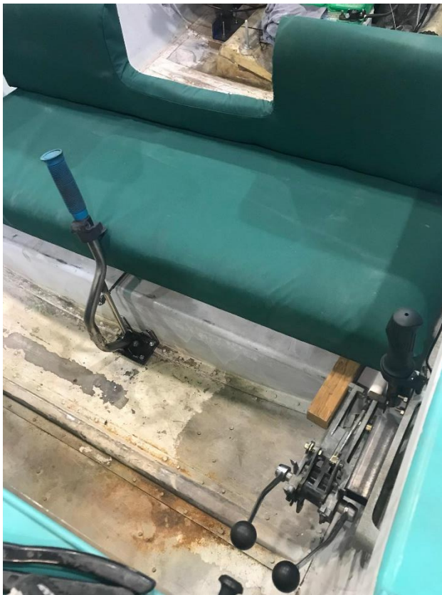
Push/Pull cable being bolted into our repurposed handlebars. A custom bracket had to be fabricated to support the handle. The bracket was riveted into the front of the front seat.
