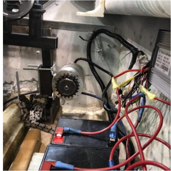
Twist grip throttle welded to angle steel and bolted to the original boat throttle mounting plate. Right picture is an alternate view of electric motor, controller, and battery packs.
