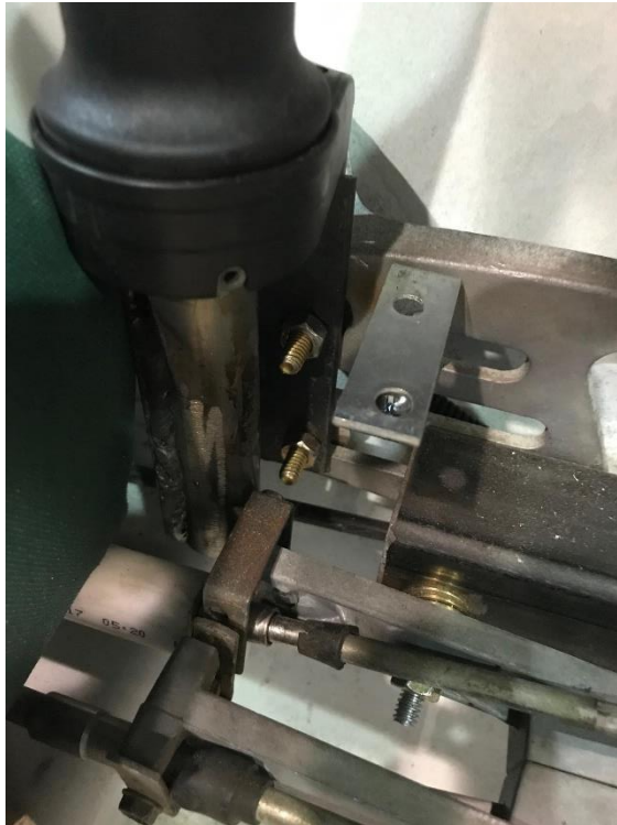
Twist grip throttle welded to angle steel and bolted to the original boat throttle mounting plate. Right picture is an alternate view of electric motor, controller, and battery packs.
