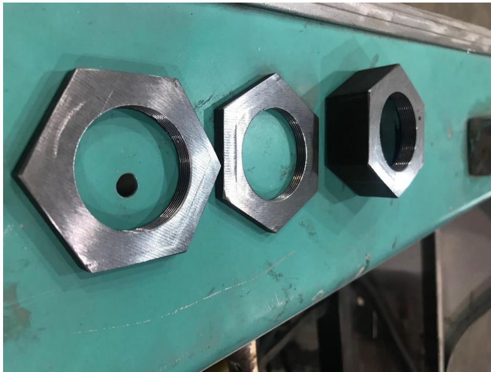
Custom made lock nuts for the sprockets and freewheels. The rare thread pitch required this since there were no lock nuts available with the same pitch.
