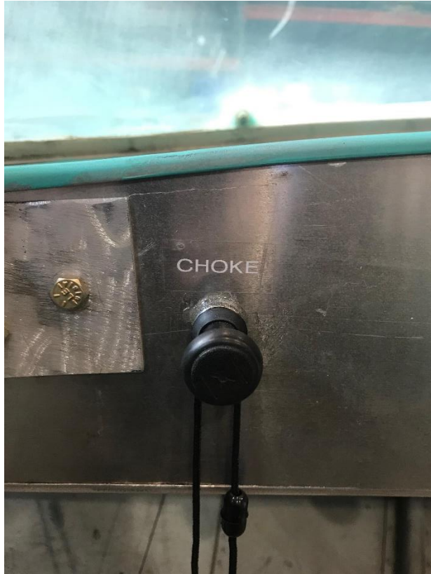
Jet ski choke control re-used and epoxied into dash. Simple pulley system used to run cable back to engine.
