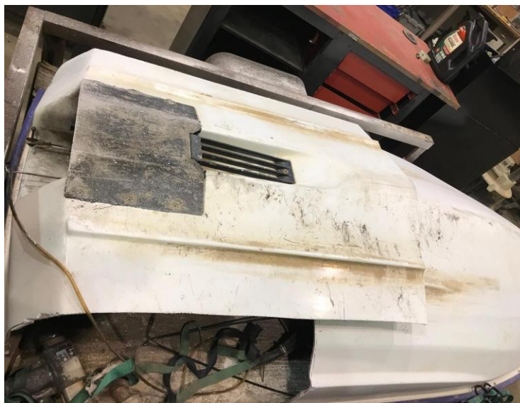
With the motor pulled we could then see how much of the jet ski hull we would need. The hull will have to be prepped for a good bond to aluminum hull.
