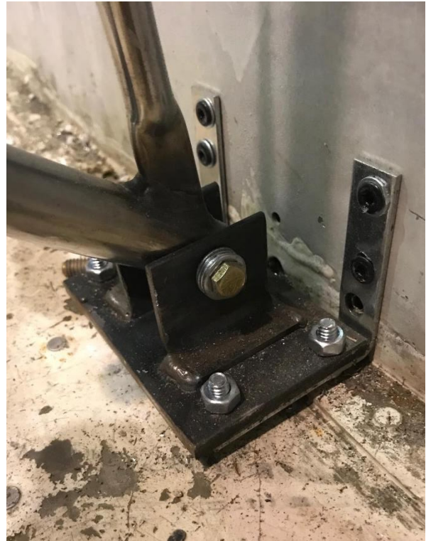
Push/Pull cable being bolted into our repurposed handlebars. A custom bracket had to be fabricated to support the handle. The bracket was riveted into the front of the front seat.
