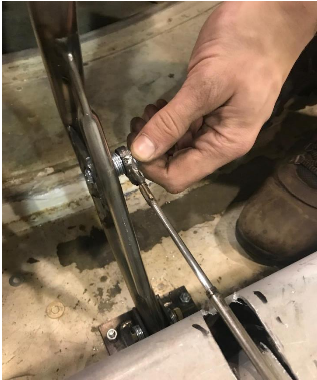
Push/Pull cable being bolted into our repurposed handlebars. A custom bracket had to be fabricated to support the handle. The bracket was riveted into the front of the front seat.
