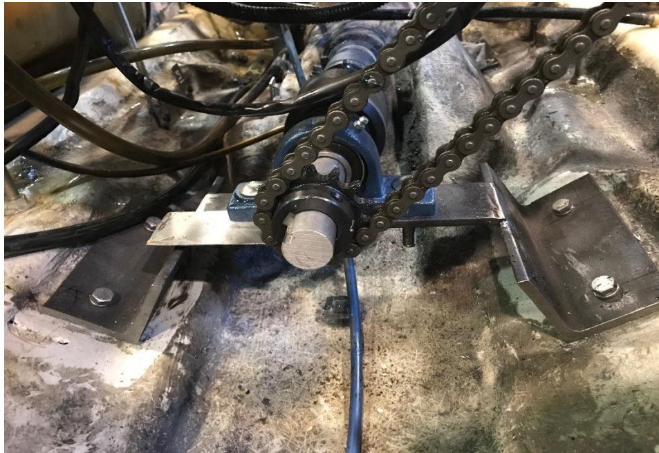
1/4" x 2 x 2 angle steel used for lower drive bearing mount.
